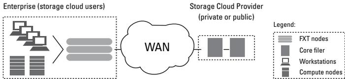
**Figure 6-4:** Both computation and the most frequently accessed storage are at the enterprise end, minimizing WAN traffic.
