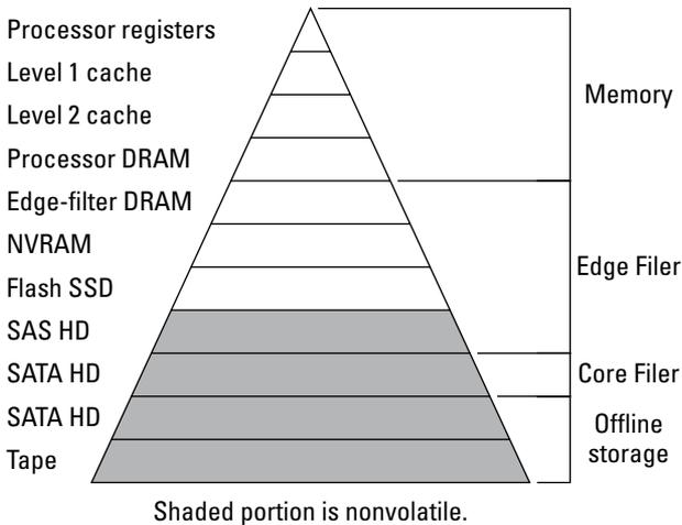
**Figure 1-2:** The expanded tiered storage model.
