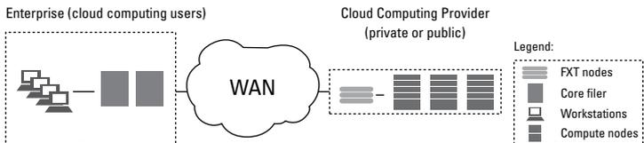
**Figure 6-2:** An Avere FXT Edge filer at the compute cloud localizes computation to the cloud, avoiding WAN latency.
