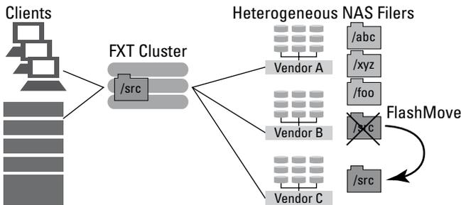
**Figure 4-1:** The FXT cluster coordinates the movement of the /src folder from Vendor B's Core filer to Vendor C's Core filer without affecting client operations.
